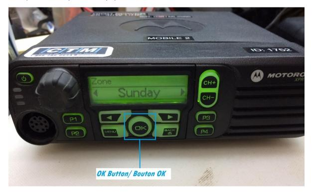
You may see Searching on the screen, just wait a few seconds. If it doesn't connect, change the channel, by pressing the channel selector button.
